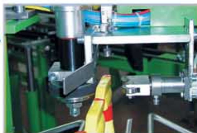
Automatic spinning with the help of lateral rollers.
