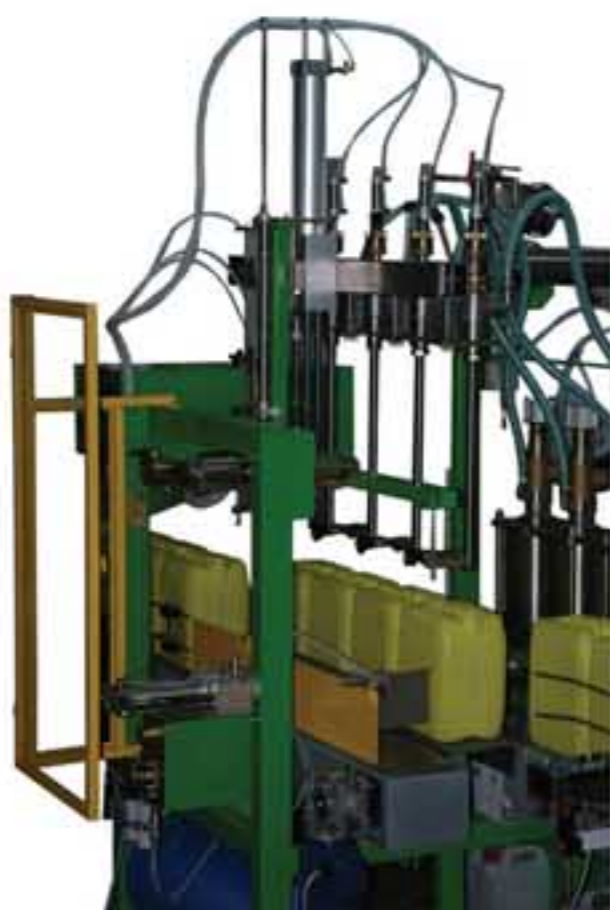
Station dosing and filling (four nozzles)
