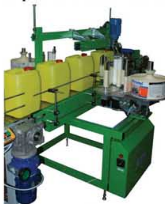
Device for labeling on two sides (Self-pasted labels in a roll)
