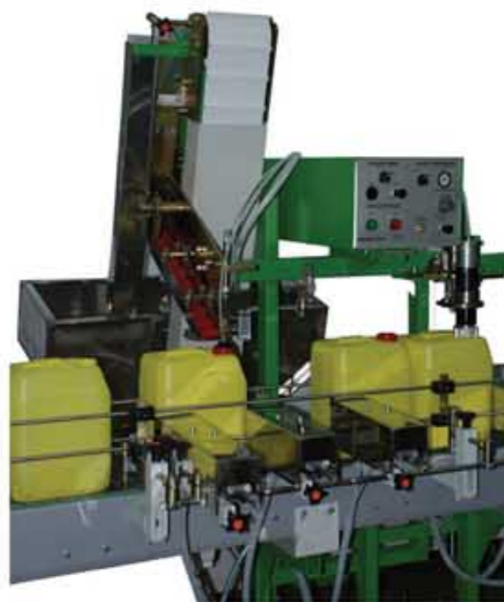
Device of automatic stacking and twisting of polyethylene covers
